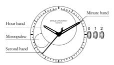
In addition to the regular functions of mechanical watch, the moon rotates clockwise a circle in 29.5 days.
