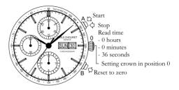
The chronograph function measures time up to 12 hours. The hourcounter measures 12 hours per rotation. The minute counter measures 30 minutes per rotation. The second counter measures 60 seconds per rotation.
